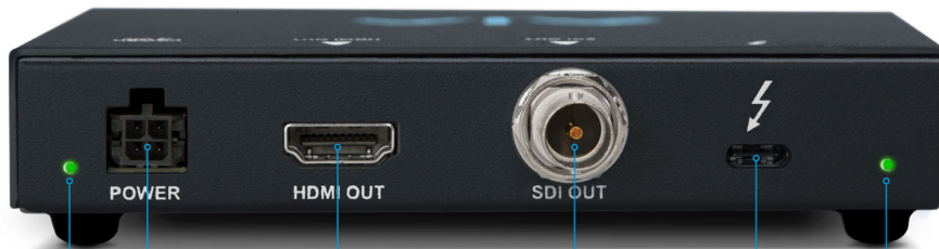
Power Light Power HDMI 2.0 Output 12G-SDI Output Thunderbolt 3 Status Light
