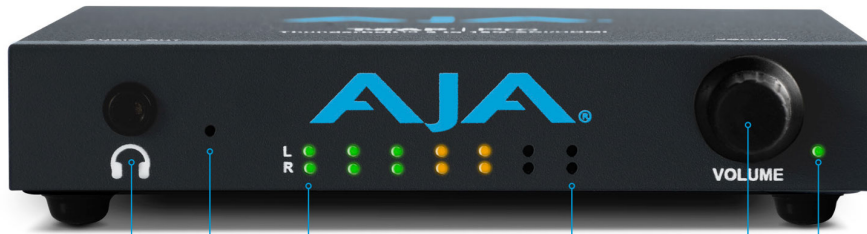
Headphone Monitor (Analog 3.5mm stereo) Safeboot Button (Recessed button) Audio Display Audio Volume/Gain Status Light
