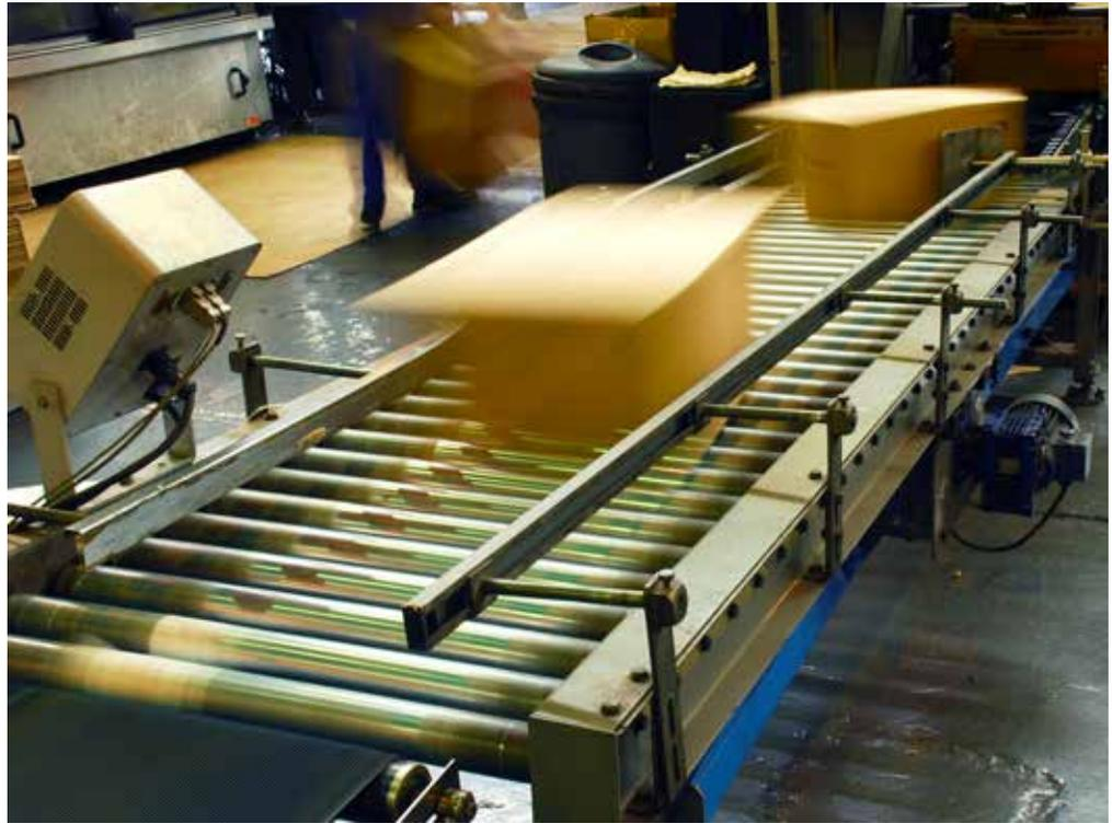
An example of machine vision application is its use for sorting letters and packages at a mail distribution center. This application uses optical character recognition (OCR) of the address label or image capture of the bar code on packages flowing down conveyer belts destined for different parts of the globe.
