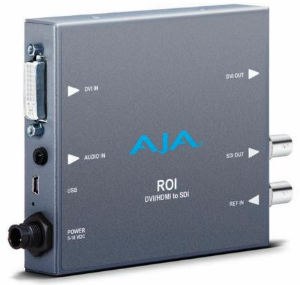
AJA's ROI Mini-Converter allows exceptionally high quality conversion of computer DVI and HDMI outputs to baseband video over SDI at an affordable price and a very portable size. With extensive audio functionality, incredible image scaling as well as aspect and frame rate conversion, ROI fulfills the growing need to properly incorporate computer signals into the video world without sacrificing budget or space.
