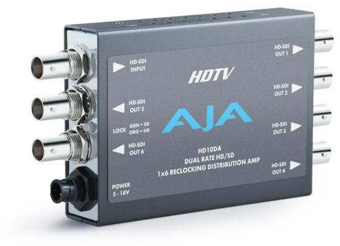
The HD10DA is a miniature, low-cost 1x6 HD/SD-SDI (dual-rate) re-clocking distribution amplifier. Featuring six separately buffered HD/SD-SDI outputs, the HD10DA provides automatic input HD cable EQ to 125 meters.
