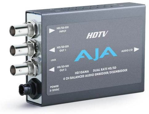
The HD10AM is a dual rate 8 channel AES audio Embedder/Disembedder. The Disembedder is always functional providing 4 AES outputs. The Embedder is user selectable, on a channel pair basis, to either "pass" SDI input audio or embed input AES audio from the breakout cable. AES inputs are sample rate converted to a 48KHz rate synchronous to the video input. The HD10AM automatically detects and configures to the input video standard. 8 x XLR breakout cable included.
