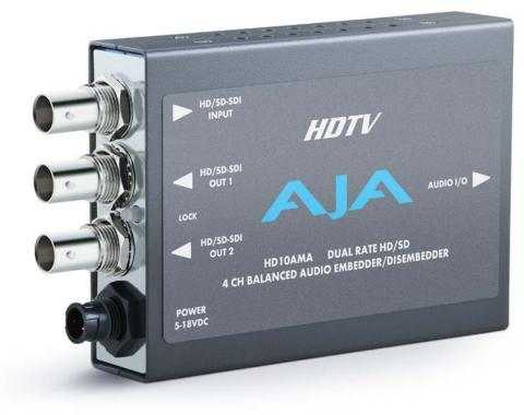
The HD10AMA is a dual rate 4 channel analog audio Embedder/Disembedder. The Disembedder is always functional providing 4 outputs. The Embedder is user selectable, on a channel pair basis, to either "pass" input audio or embed input audio from the breakout cable. Analog audio levels are selectable. The HD10AMA automatically detects and configures to the input video standard. 8 x XLR breakout cable included.
