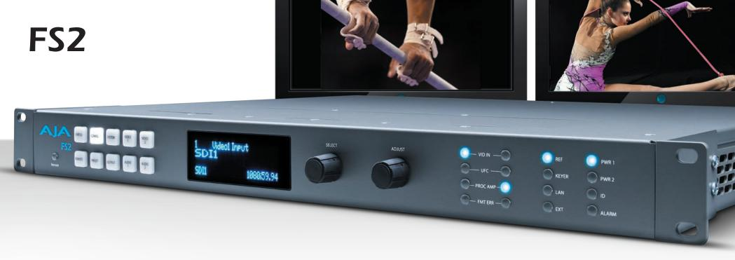
With dual-channel conversion and frame synchronizing in a slim 1RU space, FS2 can do the work of two separate devices or combine both processors together for maximum flexibility.
